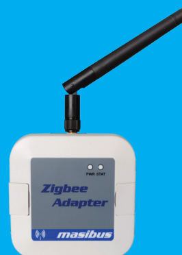
MSC-ZB-RS (RS-485 Serial to ZigBee Wireless Converters)
