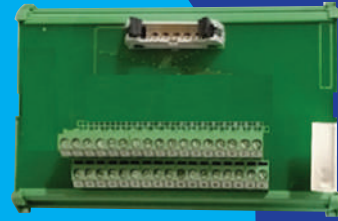
MAS-P-F25-M/MAS-P-F25-F FRC (PLC Side) to Screw Terminals (Field Side)
