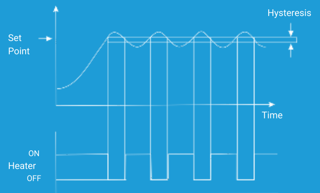
Characteristics of ON/OFF Control Action
