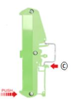
STEP 3: Remove the Module from DIN Rail as shown below
