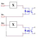
Where X = Filtering Circuit (AC Input)
