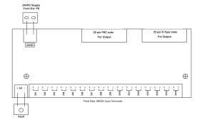
Connect rated power at terminal where 24VDC+ & 24VDC- described in wiring diagram.
