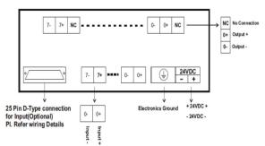
Connect rated power at terminal where 24VDC+ & 24VDC- described in wiring diagram.
